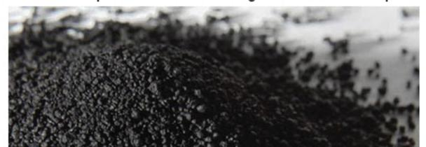
Carbon black is virtually pure elemental carbon in the form of colloidal particles that are produced by incomplete combustion or thermal decomposition of gaseous or liquid hydrocarbons under controlled conditions.
